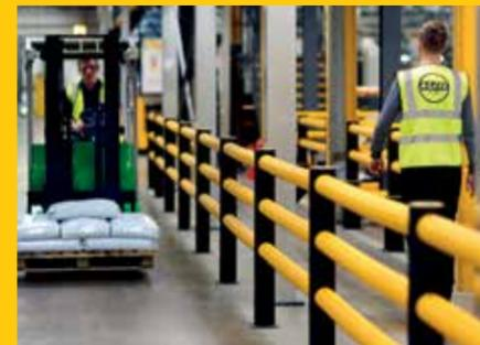
iFlex Pedestrian Guardrail separating traffic and protecting pedestrians within a factory.
